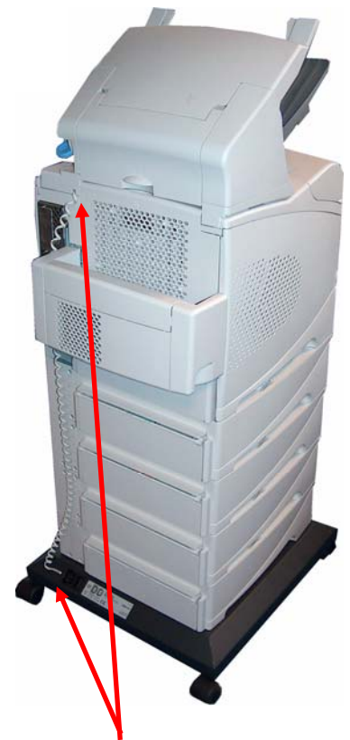
Data-Cable position on unit with stacker – arrows indicating connection socket
